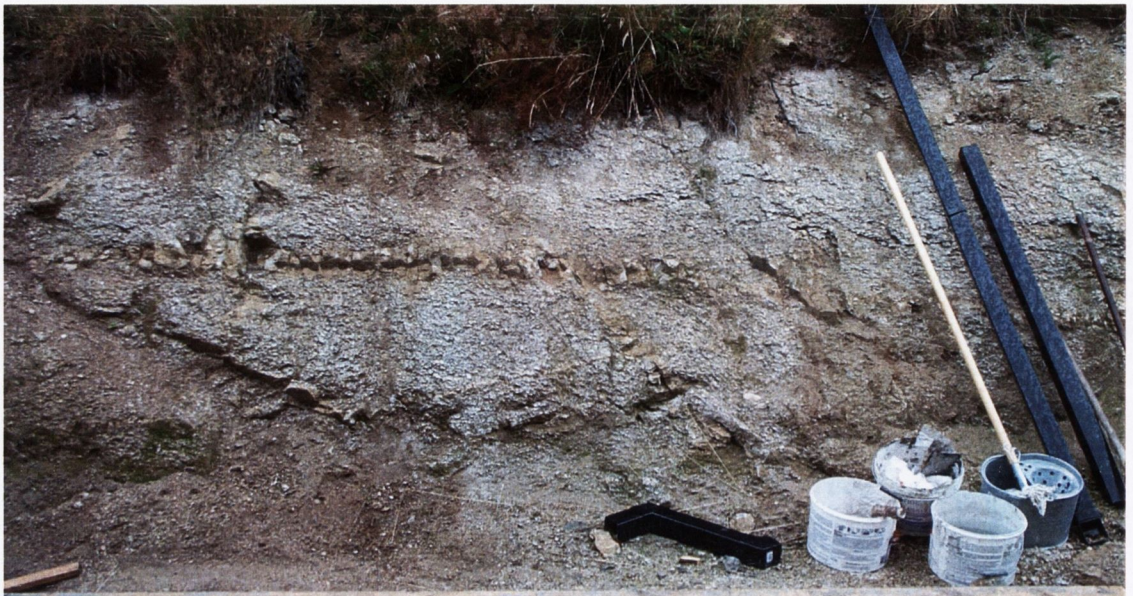
Fig. 6.2: An exposure of grus uncovered during building the foundations of house near Ballynastockan Brook, County Wicklow [302422 208779, 240m OD].
