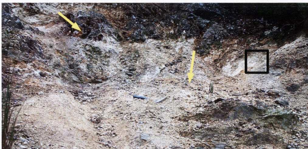
Fig. 6.12; Sample of supergene lead weathering was collected from the outcrop marked with the arrow on the left; the rusty red colour is the gossan weathering. The arrow to the right indicates the approximate location of the exit of the tepid spring in 1998, now covered by debris. The box highlights the sample location
