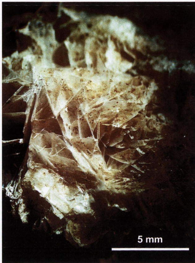
Fig. 6.13: Platy calcite collected from the spoil heaps of Glendasan, County Wicklow. Platy calcite indicates vigorous fluid boiling that caused \text{CO}_2 loss resulting in rapid mineralisation (Etoh et al. , 2002).
