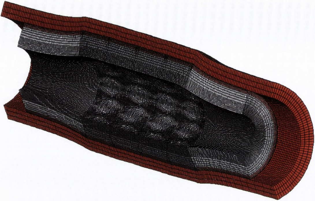
Figure 4.45 Deformed geometry of a segment of the idealised cylindrical vessel stented with the S7 stent illustrating the thrombotic layer (pink) and all of the potential restenotic growth within the lumen of the vessel (white elements).
