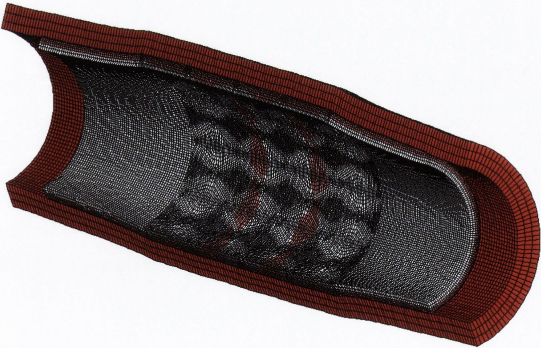
Figure 4.46 Deformed geometry of a segment of the idealised cylindrical vessel stented with the S7 stent with completely deactivated layers of potential restenotic tissue removed.
