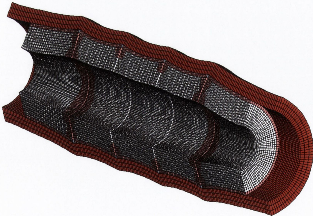
Figure 4.61 Deformed geometry of a segment of the idealised cylindrical vessel stented with the 'simple' stent with completely deactivated layers of potential restenotic tissue removed.
