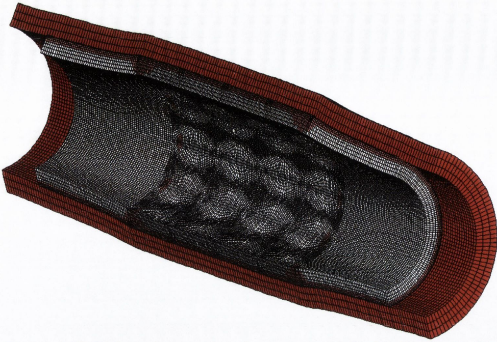
Figure 4.58 Deformed geometry of a segment of the idealised cylindrical vessel stented with the S7 stent with completely deactivated layers of potential restenotic tissue removed.
