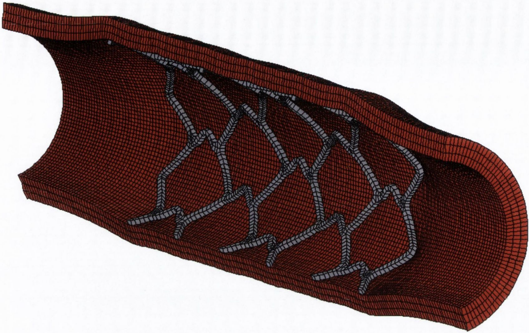
Figure 4.39 Deformed geometry of a segment of the idealised cylindrical vessel stented with the NIR stent ( \lambda_z = 1.2 ).
