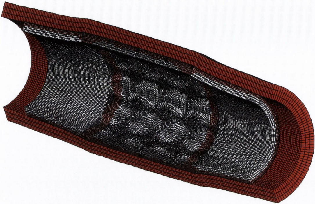
Figure 4.68 Deformed geometry of a segment of the idealised cylindrical vessel stented with the S7 stent with completely deactivated layers of potential restenotic tissue removed.
