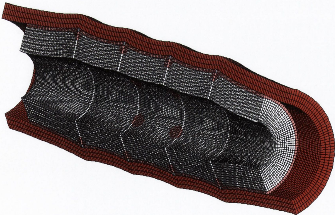
Figure 4.71 Deformed geometry of a segment of the idealised cylindrical vessel stented with the 'simple' stent with completely deactivated layers of potential restenotic tissue removed.
