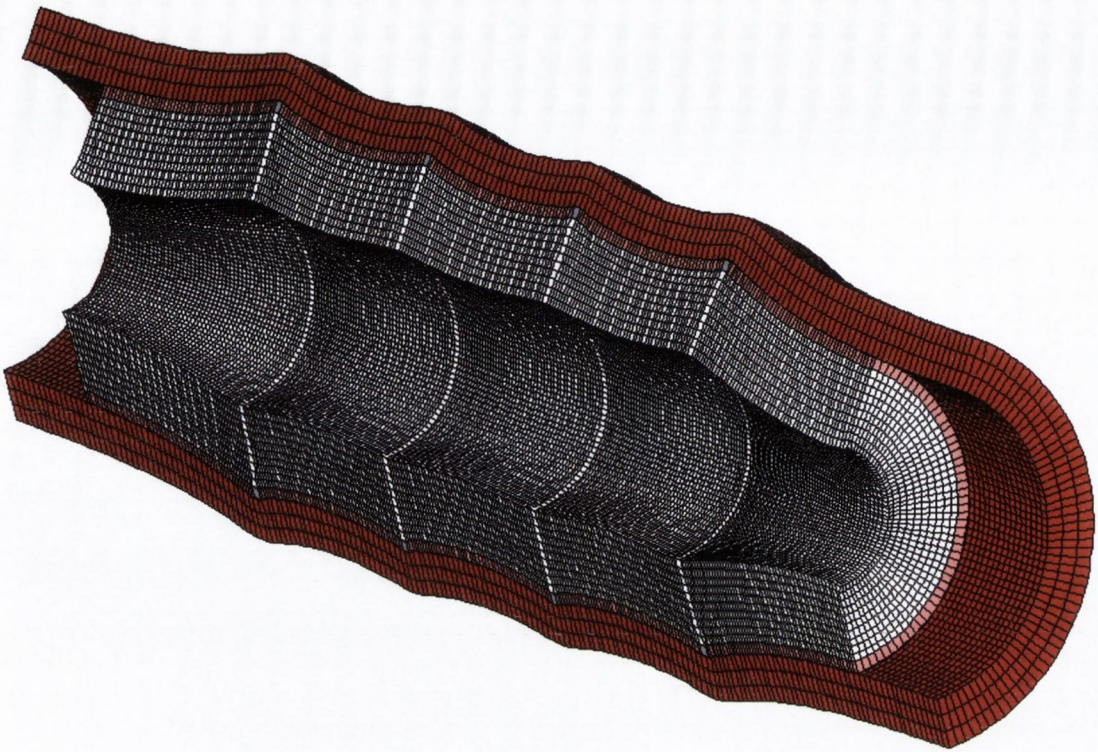
Figure 4.50 Deformed geometry of a segment of the idealised cylindrical vessel stented with the S7 stent illustrating the thrombotic layer (pink) and all of the potential restenotic growth within the lumen of the vessel (white elements).
