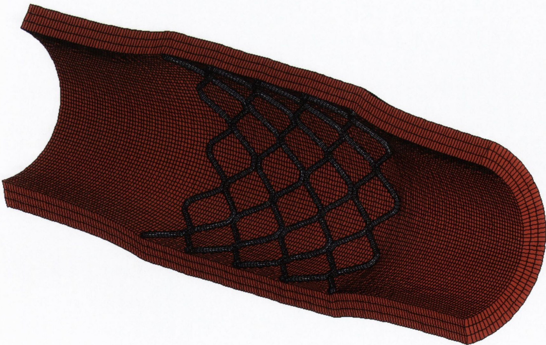
Figure 4.44 Deformed geometry of a segment of the idealised cylindrical vessel stented with the S7 stent ( \lambda_z = 1.2 ).
