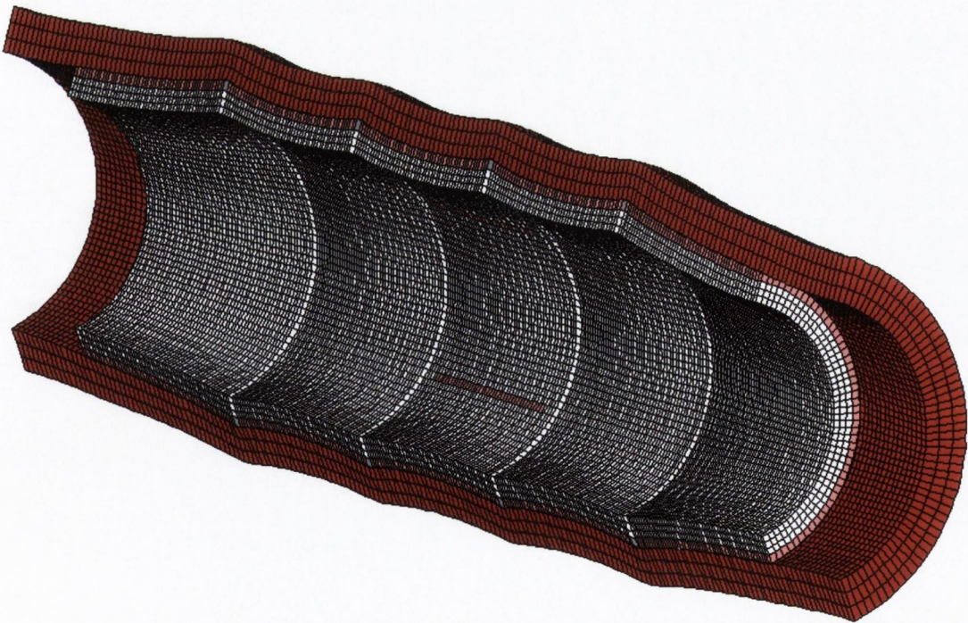
Figure 4.51 Deformed geometry of a segment of the idealised cylindrical vessel stented with the 'simple' stent with completely deactivated layers of potential restenotic tissue removed.
