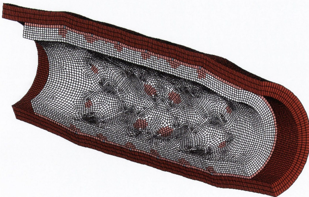
Figure 4.65 Deformed geometry of a segment of the idealised cylindrical vessel stented with the NIR stent with completely deactivated layers of potential restenotic tissue removed.
