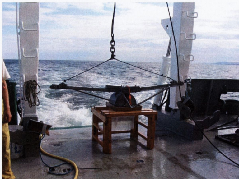
Figure 2.1: The modified long-arm continuous warp 0.1m 2 Van Veen grab onboard the RV Celtic Voyager, July 2005.
