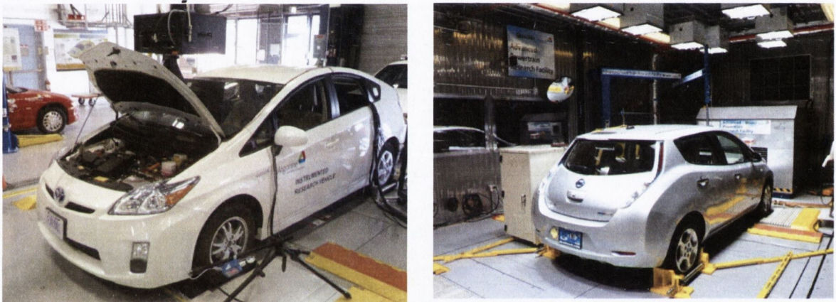
Figure 4.1. Images of the dynamometer testing of vehicles (Rask and Rousseau, 2012).
