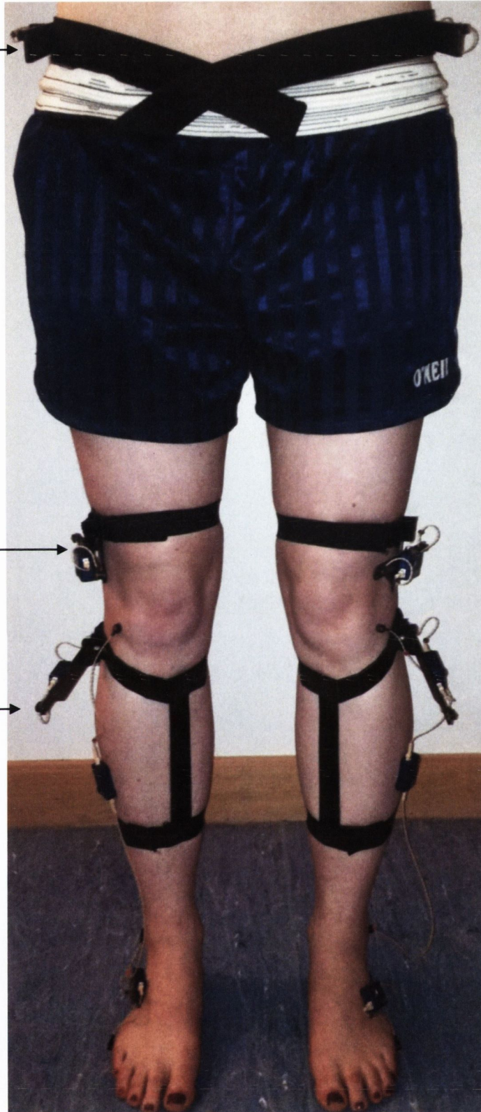
Figure 3.9: Bilateral gait LED application (front view).
