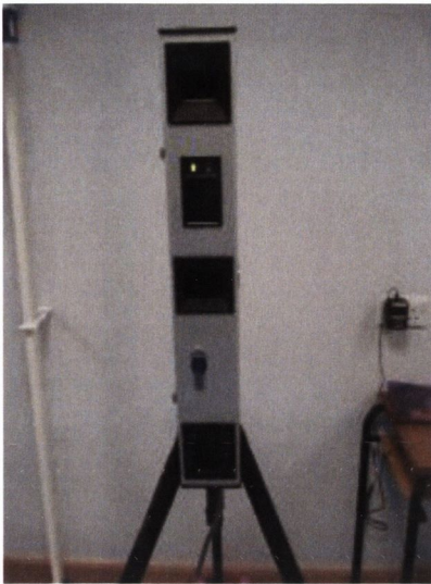
Figure 3.2: CODA motion sensor.
