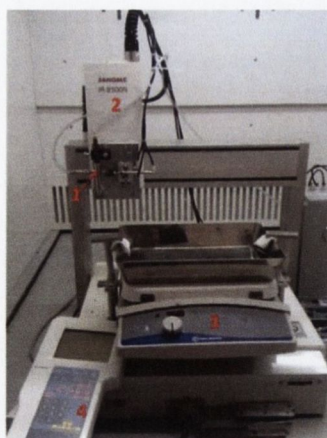
Figure 4.18 Spray set up of the Janome JR 2300N automatic robot showing; 1: airbrush with compressed air feed attached 2: mechanical robot with pneumatic arm 3: hotplate where substrate is placed 4: programmable controller.
