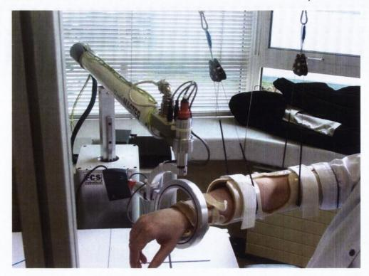
Figure 4-8. Arm attachment to the GENTLE/s system
