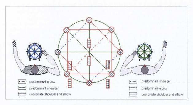
Figure 3-2, Patterns of movement of MIT Manus robot
