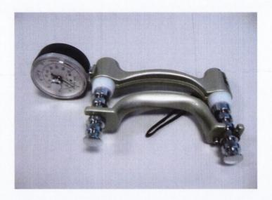
Figure 4-6. Jamar hand-held dynamometer
