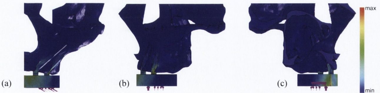
Figure 6.21 – Model 7 under 30° palatal loading: (a) anterior, (b) lateral and (c) medial views.
