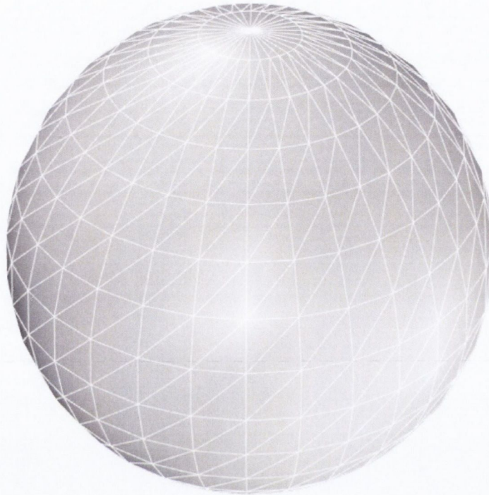
Figure 4.11 - An STL model of a sphere
