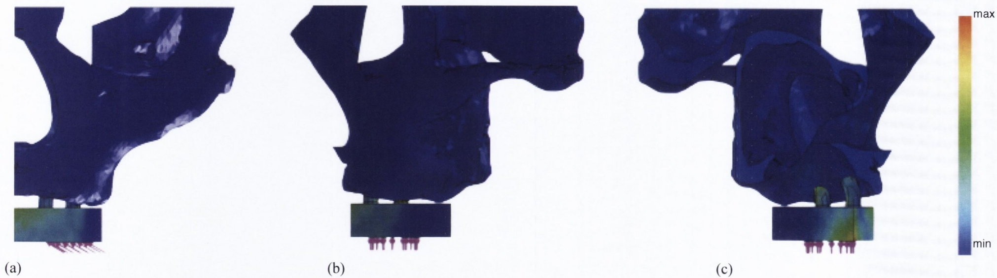
Figure 6.12 – Model 4 under 30° palatal loading: (a) anterior, (b) lateral and (c) medial views.
