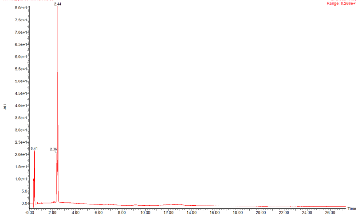
Figure 5: 100 ppm Each of nifedipine, impurity A and impurity B. Mobile phase: water/acetonitrile (65:35) with 0.1% formic acid. Column temperature 35°C. Flow rate: 0.4 mL/min. Injection: 8 \mu L.
