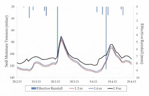
Figure 7.34 Soil moisture response to effective rainfall beneath LPP at Site B
