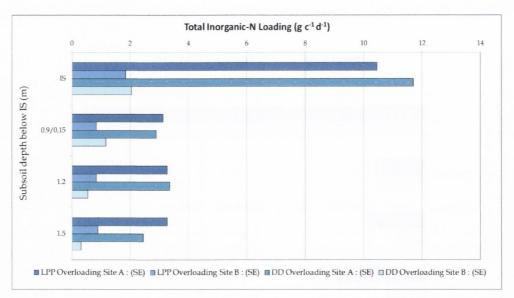
Figure 8.16 Mean Inorg-N load per capita at the designated depth planes beneath the LPP and DD
