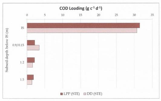
Figure 8.5 Mean COD load per capita at the designated depth planes beneath the LPP and DD
