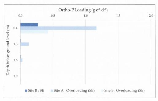
Figure 8.18 Mean Ortho-P load per capita at the designated depth planes beneath LPP (SE)
