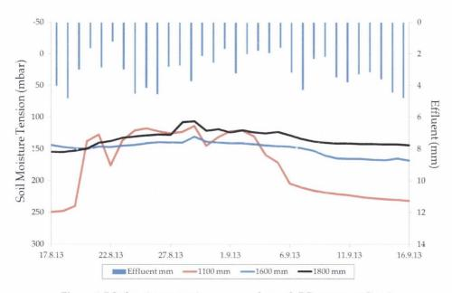
Figure 1.7 Soil moisture tension response beneath DD system at Site A
