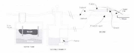
Figure 2.10 Cross-section of a septic tank mound system for on-site wastewater disposal (adapted from Converse et al. (1978))
