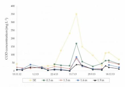
Figure 7.56 Reduction in COD load with respect to the SE at all depth planes
