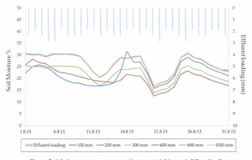
Figure 7.40 Soil moisture response to effective rainfall beneath DD at Site B  $\,$
