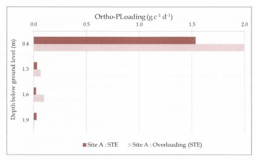
Figure 8.17 Mean Ortho-P load per capita at the designated depth planes beneath LPP (STE)
