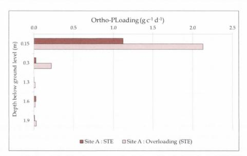
Figure 8.19 Mean Ortho-P load per capita at the designated depth planes beneath DD (STE)
