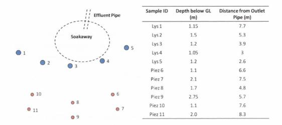
Figure 4.8 Instrumentation layout of Site C
