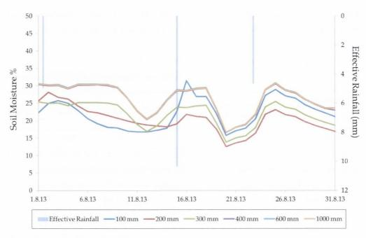
Figure 7.39 Soil moisture response to effective rainfall beneath DD at Site B  $\,$
