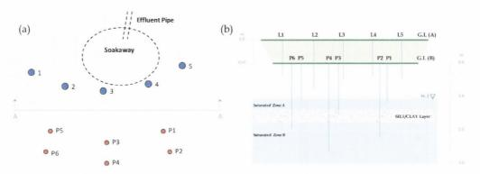
Figure 6.32 (a) Plan view and (b) A-A cross-section of installed instrumentation at Site C
