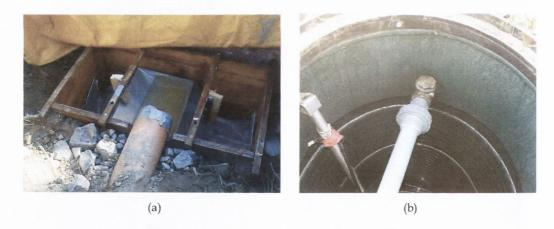
Figure 4.23 (a) Tipping bucket at Site A and (b) Orpheus mini level sensor at Site B
