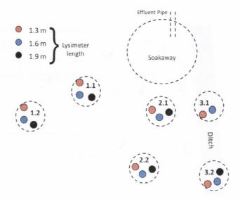
Figure 6.1 Plan of instrumentation at Site A (pre-remediation)
