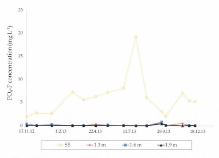
Figure 7.55 Reduction in PO<sub>4</sub>-P load with respect to the SE at all depth planes
