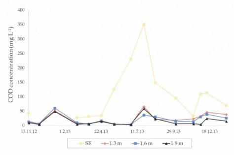
Figure 7.53 Reduction in COD with respect to SE at all depth planes
