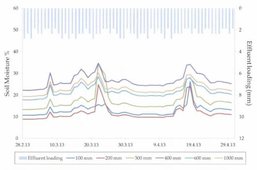
Figure 7.33 Soil moisture response to effective rainfall beneath LPP at Site B
