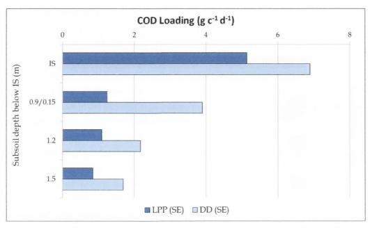
Figure 8.7 Mean COD load per capita at the designated depth planes beneath the LPP and DD
