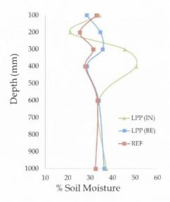
Figure 7.31 Mean soil moisture variation with depth beneath LPP system at Site B
