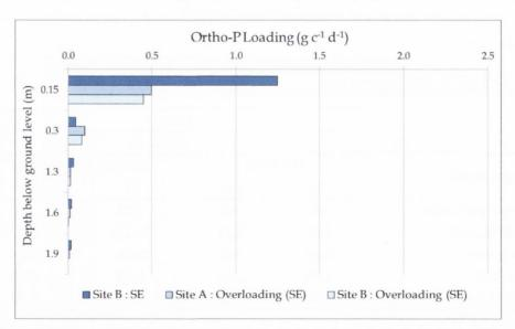
Figure 8.20 Mean Ortho-P load per capita at the designated depth planes beneath DD (SE)
