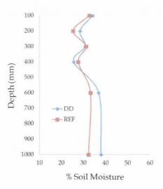
Figure 7.38 Soil moisture variation with depth beneath DD system at Site B
