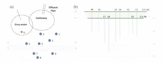
Figure 6.47 (a) Plan view and (b) A-A cross-section of installed instrumentation at Site D
