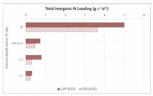
Figure 8.13 Mean Inorg-N load per capita at the designated depth planes beneath the LPP and DD
