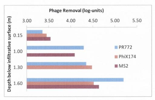
Figure 7.62 Phage log-unit removal recorded at each depth plane at all sample positions over the duration of the trial
