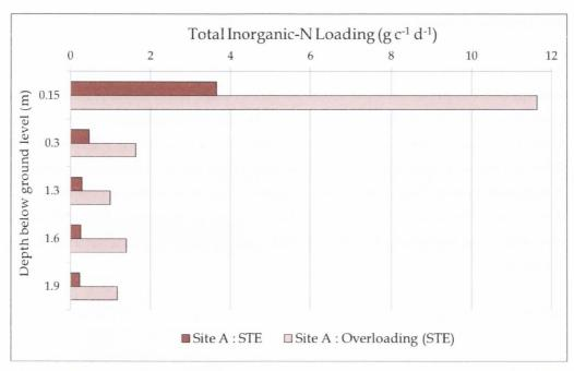
Figure 8.11 Mean Total Inorg-N load per capita at the designated depth planes beneath DD (STE)
