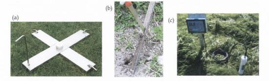
**Figure 4.30** (a) soil moisture stabilisation plate, (b) soil moisture auger and (c) installed soil moisture probe and data logger
