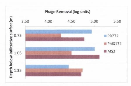
Figure 7.61 Phage log-unit removal recorded at each depth plane at all sample positions over the duration of the trial
