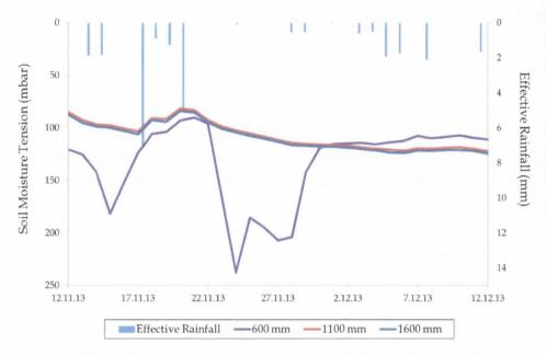
Figure 1.16 Soil moisture tension response to effective rainfall at Site B
