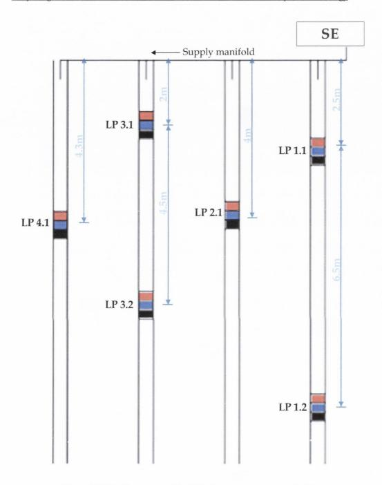
Figure 4.27 Labelling sequence for LPP soil moisture samples at Site B
