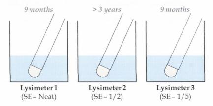
Figure 1 Testing apparatus showing dilution factors and age of lysimeters
