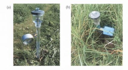
Figure 4.29 (a) Jet Fill Tensiometer and (b) data logging tensiometer
