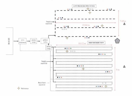
Figure 4.17 Overall setup at Site B
