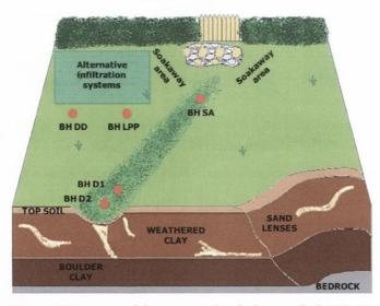
Figure 4.6 Locations of downstream boreholes installed at Site B
