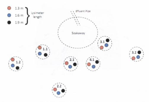
Figure 4.5 Instrumentation layout at Site B
