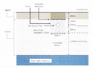
Figure 2.9 Section of a conventional percolation trench receiving STE (EPA, 2009a)
