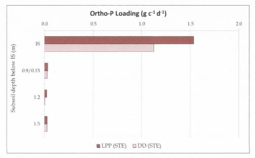
Figure 8.21 Mean Ortho-P load per capita at the designated depth planes beneath the LPP and DD
