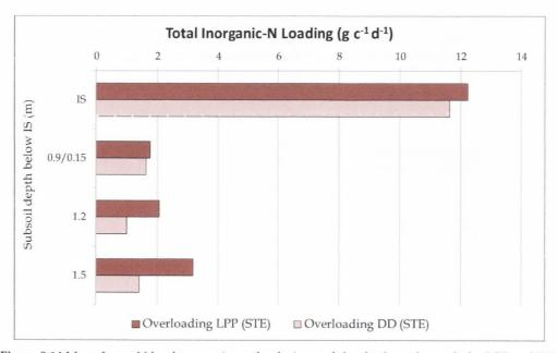
Figure 8.14 Mean Inorg-N load per capita at the designated depth planes beneath the LPP and DD
