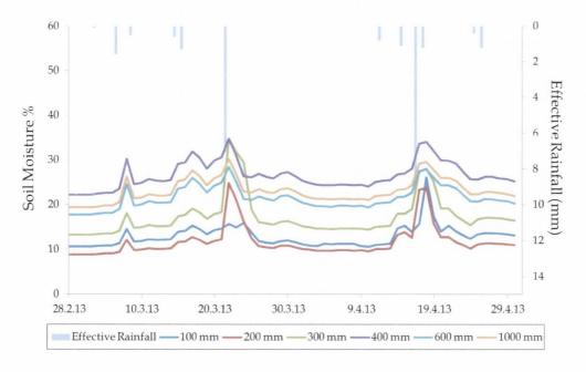
Figure 7.32 Soil moisture response to effective rainfall beneath LPP at Site B
