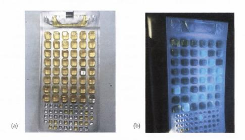
Figure 4.33 Positive readings for (a) Total coliforms and (b) E. coli
