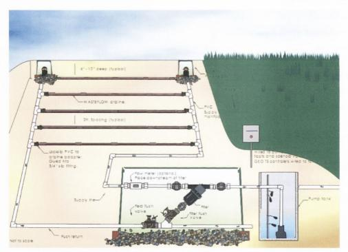
Figure 2.11 Typical drip field layout for a individual instalment (Geoflow, 2007)
