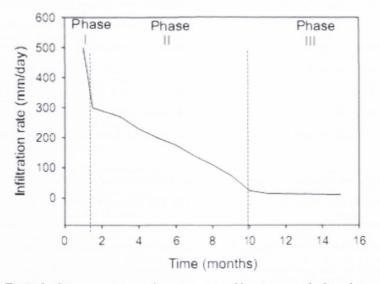
Figure 2.4 Typical schematic pattern of wastewater infiltration rate decline through infiltrative surface over time (Beal 2005 (from Otis 1984))
