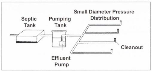
Figure 2.12 Low pressure pipe system (USEPA (1992); cited by USEPA (1999))
