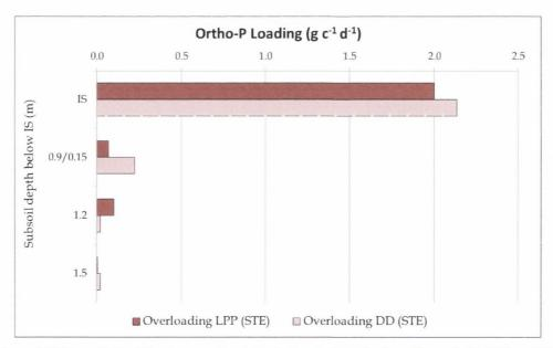
Figure 8.22 Mean Ortho-P load per capita at the designated depth planes beneath the LPP and DD
