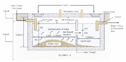
Figure 2.2 Longitudinal section of typical two-chamber septic tank (EPA, 2009a)
