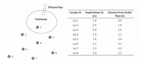
Figure 4.14 Instrumentation layout at Site F
