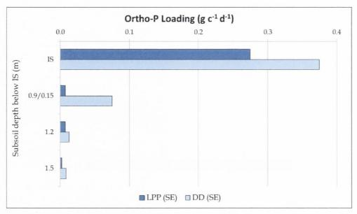
Figure 8.23 Mean Ortho-P load per capita at the designated depth planes beneath the LPP and DD
