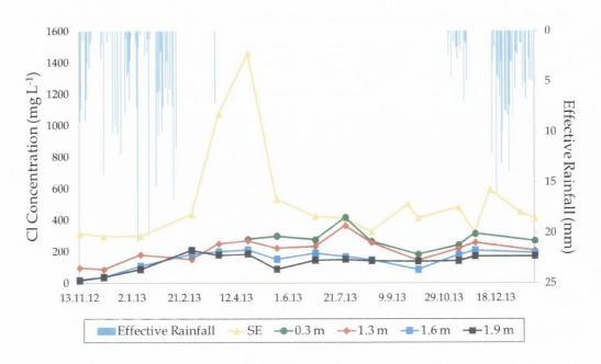
Figure 7.36 Effect of dilution by ERF on Cl concentrations beneath DD system at Site B
