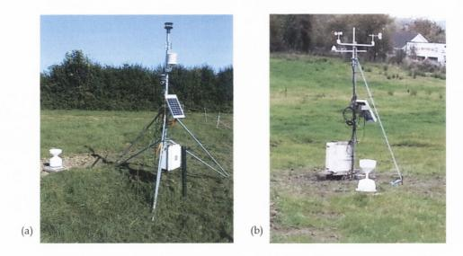
Figure 4.32 Weather stations installed at (a) Site A - Kilkenny and (b) Site B - Monaghan
