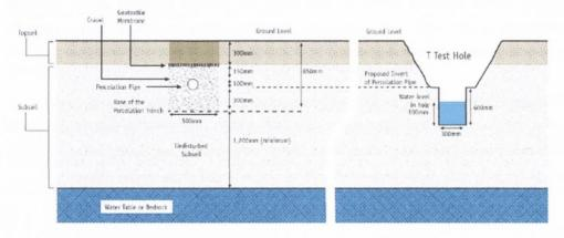
Figure 3.1 Cross-section of a T test hole (EPA, 2009a)
