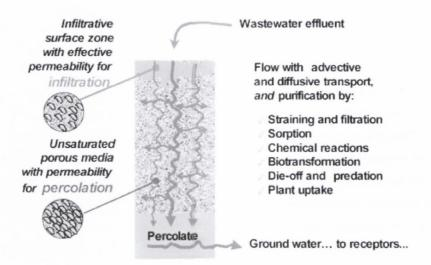
Figure 2.3 Illustration of hydraulic and purification processes operative during wastewater infiltration and percolation in soil-based systems (Van Cuyk et al., 2001)
