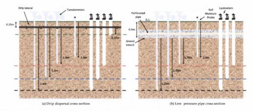
**Figure 7.1** Cross-section of instrumentation installed beneath (a) DD system and (b) LPP system at Sites A and B
