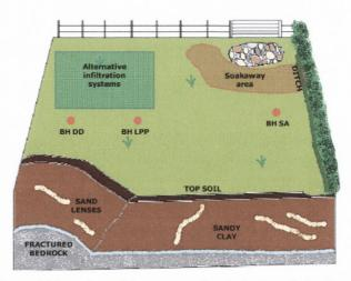
Figure 4.3 Locations of downstream boreholes installed at Site A
