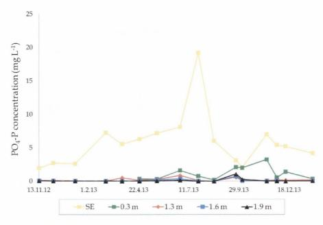
Figure 7.58 Reduction in PO<sub>4</sub>-P load with respect to the SE at all depth planes
