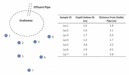
Figure 4.12 Instrumentation layout at Site E
