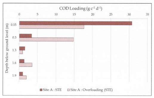
Figure 8.3 Mean COD load per capita at the designated depth planes beneath DD (STE)
