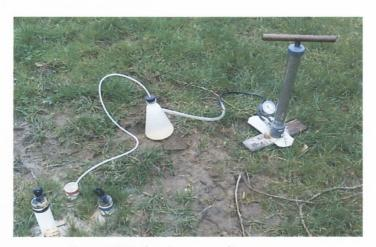
Figure 4.24 Soil moisture sampling apparatus
