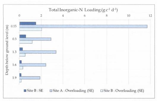
Figure 8.12 Mean Total Inorg-N load per capita at the designated depth planes beneath DD (SE)
