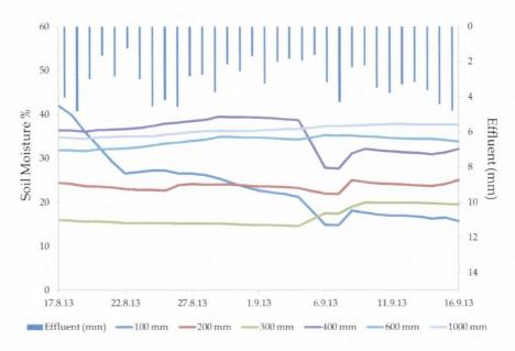
Figure 1.6 Soil moisture variation in response to effluent loading at Site A
