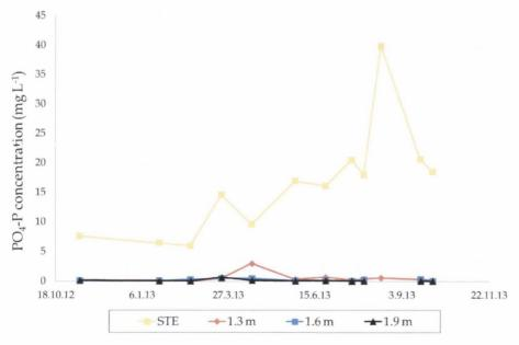
Figure 7.47 Reduction in PO<sub>4</sub>-P with respect to STE
