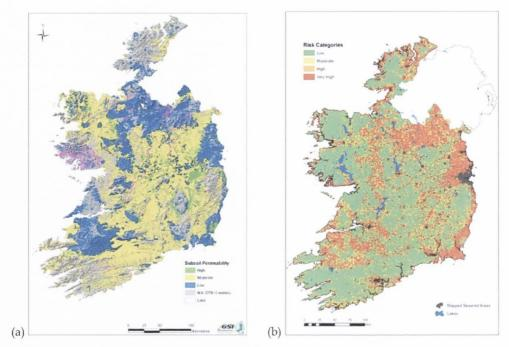
**Figure 2.7** (a) Subsoil permeability map showing different permeability classes across the Irish landmass (Meehan, 2012); (b) Relative risk of water pollution (streams) from OSWTS via surface pathway (EPA, 2012).
