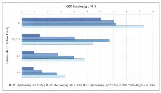
Figure 8.8 Mean COD load per capita at the designated depth planes beneath the LPP and DD
