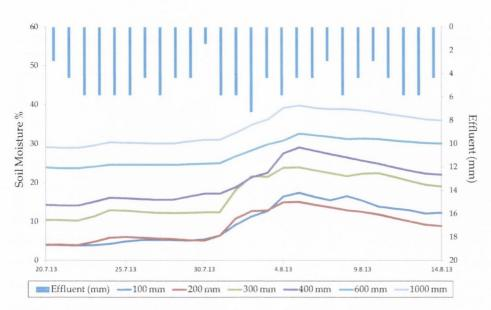
Figure 1.1 Soil moisture response to increase in effluent application
