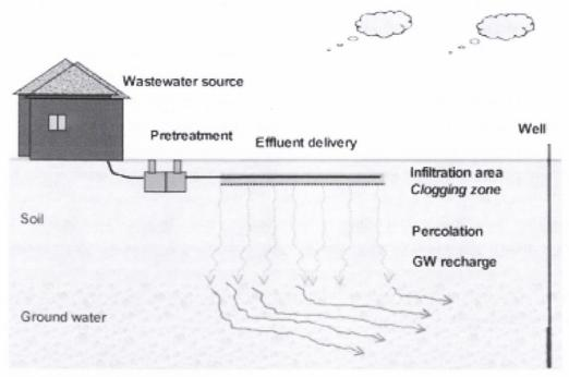
**Figure 2.1** Conventional septic tank treatment system including percolation area with pathway for potential contaminant migration to groundwater (adapted from Van Cuyk et al. (2001))
