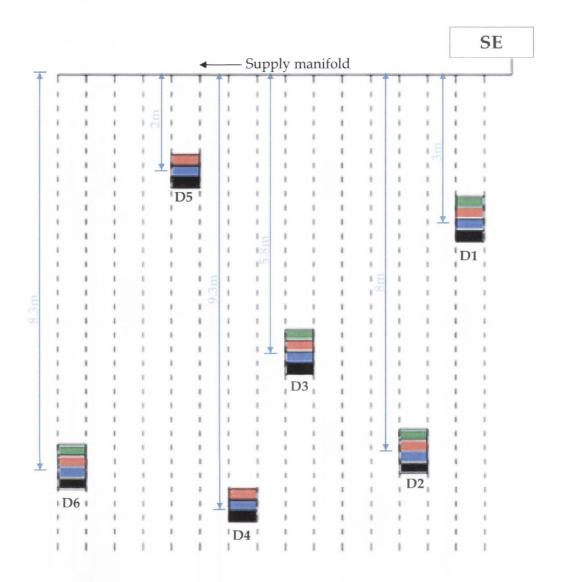
Figure 4.28 Labelling sequence for DD soil moisture samples at Site B
