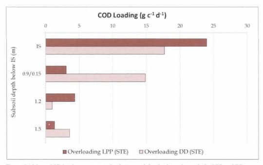
Figure 8.6 Mean COD load per capita at the designated depth planes beneath the LPP and DD
