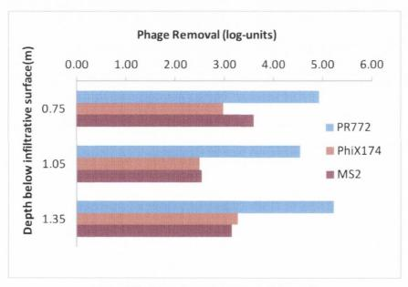
Figure 7.59 Phage log-unit removal with depth
