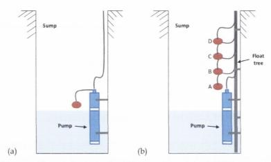
Figure 4.15 Float configuration for (a) LPP pump sump and (b) DD pump sump
