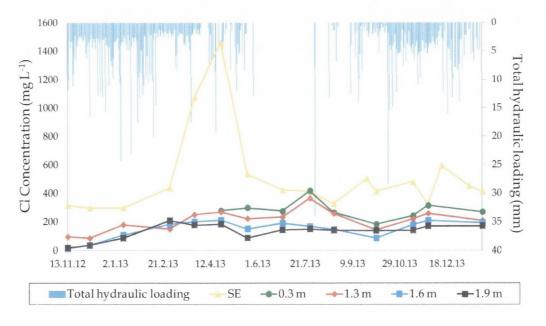
Figure 7.37 Cl concentrations against total hydraulic loading beneath DD system at Site B
