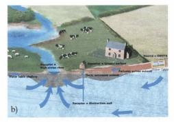
Figure 1.1 Transport of contaminants to groundwater and surface water bodies in a) areas of high permeability and b) areas of low permeability (EPA, 2012)
