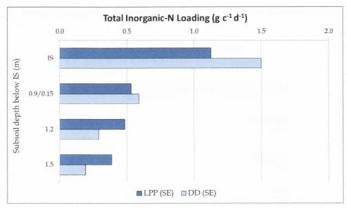
Figure 8.15 Mean Inorg-N load per capita at the designated depth planes beneath the LPP and DD
