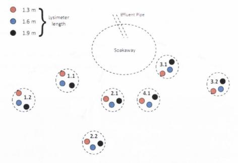
Figure 6.18 Instrumentation layout at Site B
