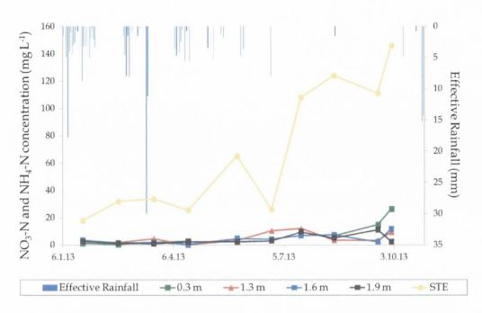
Figure 7.51 Reduction in NO<sub>3</sub>-N concentrations at all depth planes in relation to STE NH<sub>4</sub>-N concentrations and effective rainfall
