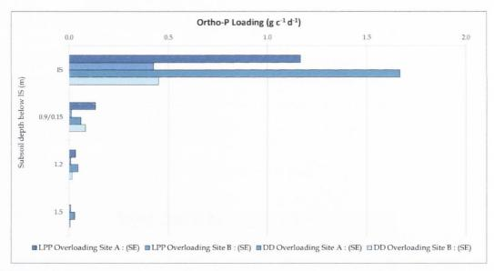
Figure 8.24 Mean Ortho-P load per capita at the designated depth planes beneath the LPP and DD
