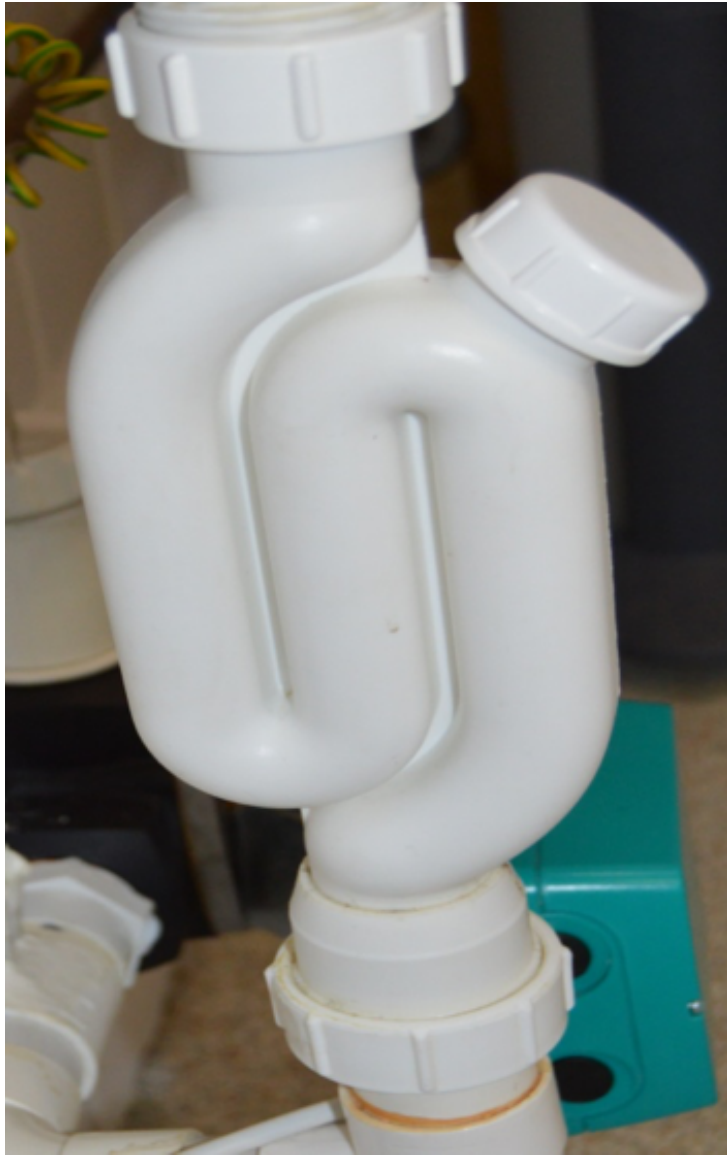
Figure 2.2 A photograph showing an example of a Multikwik polypropylene U-bend. This is the U-bend used with the automated ECA U-bend decontamination system developed in the present study. The U-bend is connected directly below the washbasin drain outlet. The sampling port visible in the upper right portion of the photograph can be unscrewed easily for taking swab samples.
