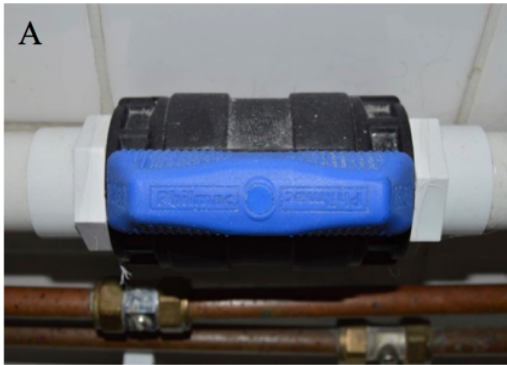
Figure 3.1 Photograph showing a manual valve fitted to a test washbasin wastewater outflow pipe downstream of the U-bend. In position (A) the valve is open and allows liquid to flow. In position (B) the valve is in the closed position and prevents liquid flowing.
