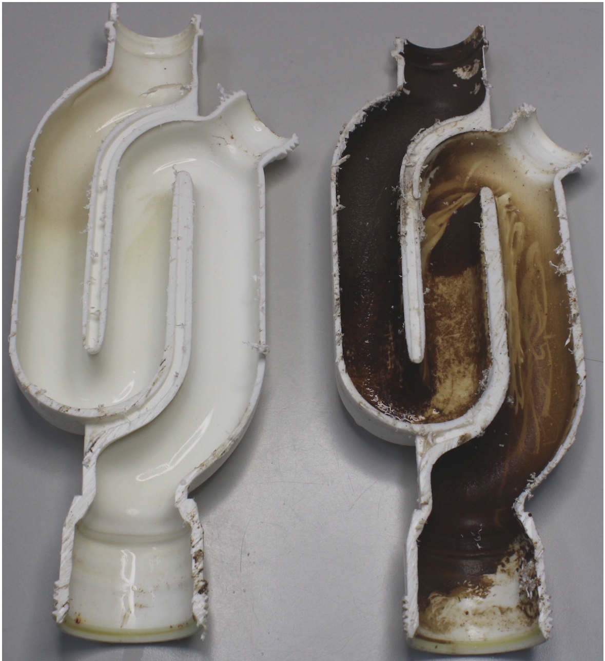
Figure 3.10 Photograph showing cross-sections of the ECA-treated (left) and control (right) U-bends used during automated washbasin U-bend decontamination. The ECA-treated U-bend was subjected to 35 cycles of treatment with catholyte for 5 min followed by anolyte treatment for 5 min over three months using the second prototype automated U-bend decontamination system developed during the study. ECA treatment cycles were undertaken three times a week on Mondays, Wednesdays and Fridays. The control U-bend was not treated with ECA-solutions. Both U-bends were fitted at the same time to identical washbasins in adjacent bathrooms. The control U-bend is heavily fouled with dense pigmented microbial biofilm. In contrast, the ECA-treated U-bend is virtually free of biofilm. These findings are supported by electron microscopy of internal sections of both U-bends (see Figure 3.11).
