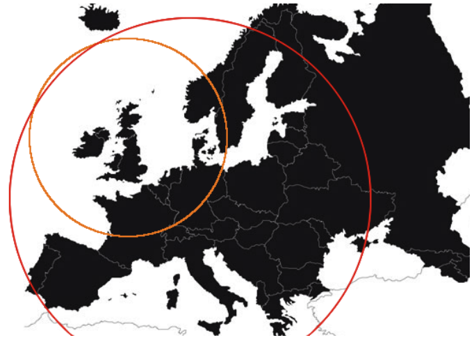
Fig. 1. This map roughly represents the area within which the MSF60 (orange) and the DCF77 (red) can be clearly received. This are the values reported by the documentation provided by the organizations responsible for the maintenance of the time signal broadcasts. However by our experience, using a cheap receiver, in Ireland the DCF77 signal is received with a lot of noise. For this reason our experiments are based on the MSF60 signal, which due to the geographical proximity of the transmitter, was received without any noise by our cheap receivers.
