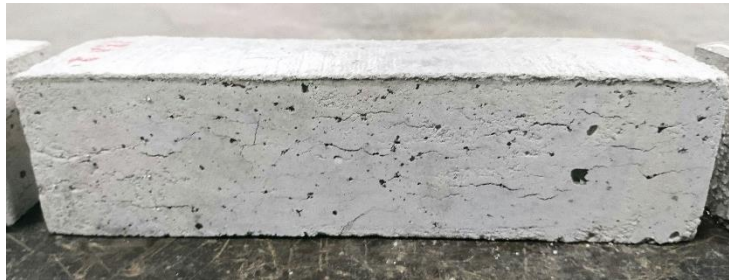
Figure 1. The ashes slightly alter the lime mortar colour (prisms used for flexural strength testing).
