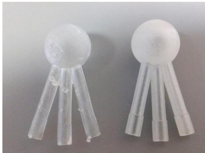
Figure A1.1: Photograph of prototype mixing chambers produced using (left) the Form1+ (Formlabs, USA) system and (right) the Eden 250 (Stratasys, USA) system.
