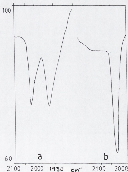
Fig.25 : IR spectra of [\text{Ru}(\text{bpy})_2(\text{CO})\text{H}][\text{PF}_6] in Nafion after treatment in \text{H}_2\text{O} for a. 30 mins and b. 90 mins
