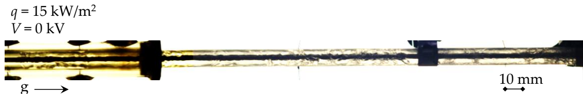
Figure 5.4 - Thermosyphon operation with no EHD forces, q = 15 \text{ kW/m}^2
