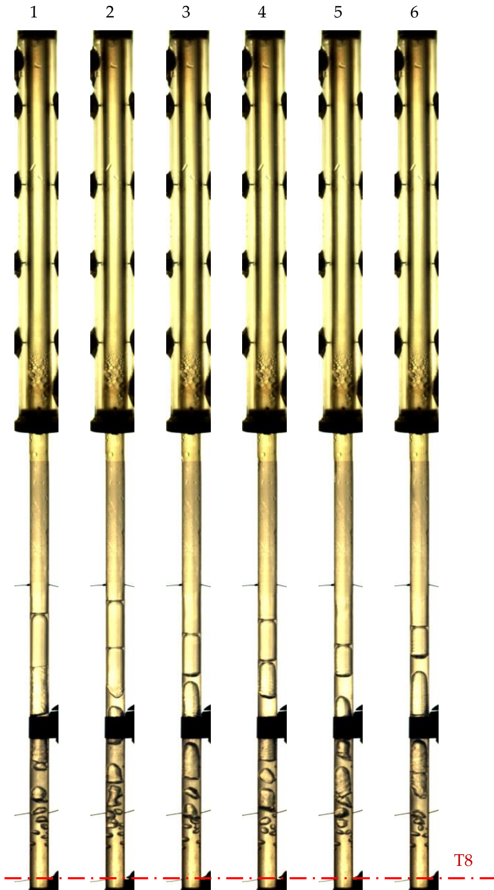
Figure 4.16 - Water at high pressure, P_r = 0.06 , q = 5.5 \text{ kW/m}^2 , \Delta t = 0.06 \text{ s}
