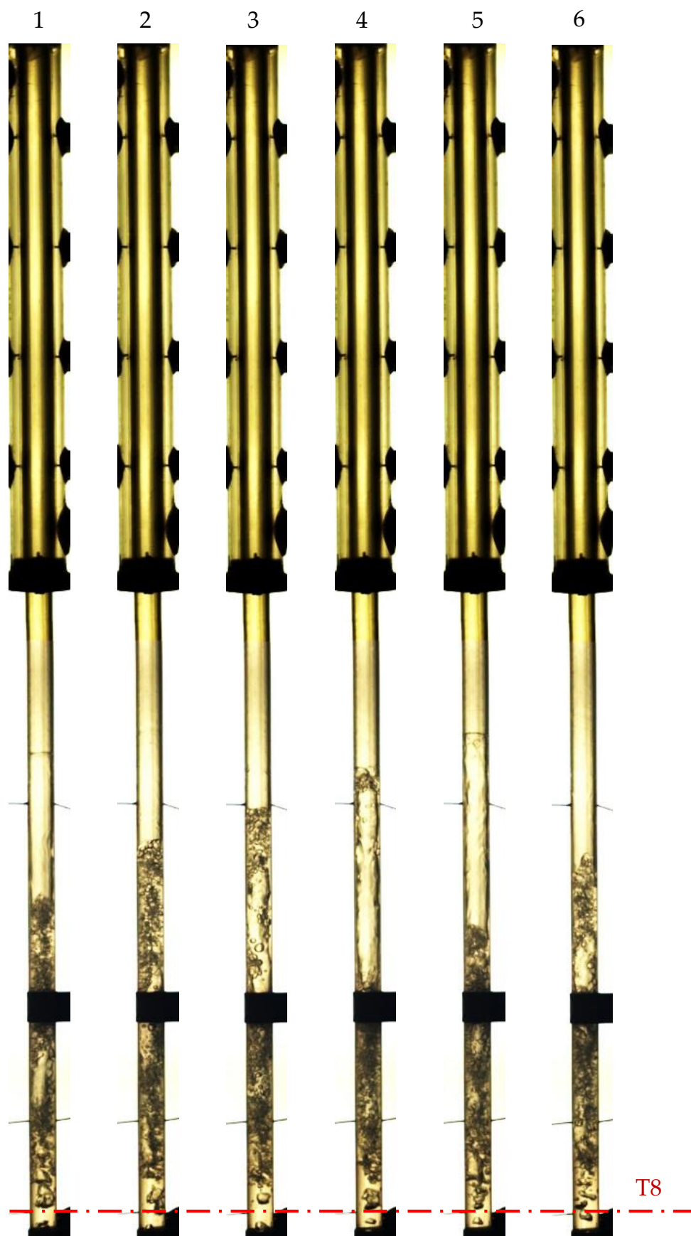
Figure 4.22 - HFE-7000, P_r = 0.06 , q = 7.8 \text{ kW/m}^2 , \Delta t = 0.06 \text{ s}
