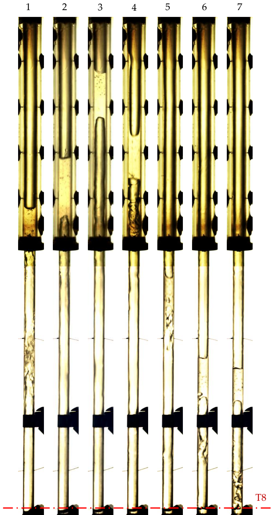
Figure 4.12 - Water, Pr = 0.0002 , q = 39 \text{ kW/m}^2 , \Delta t = 0.06 \text{ s}
