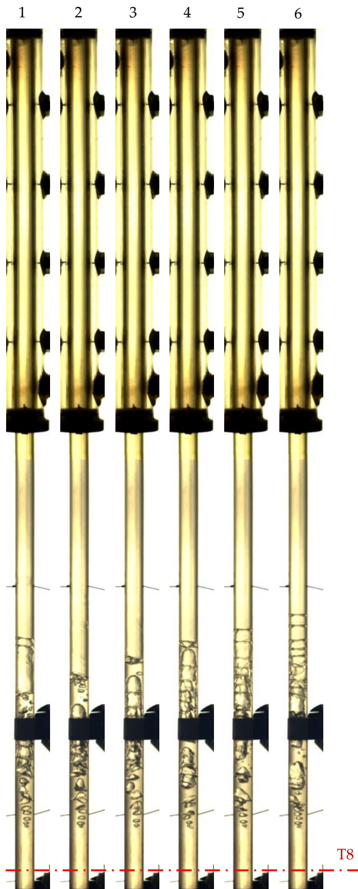
Figure 4.36 - Ethanol, Pr = 0.02 , q = 5.6 \text{ kW/m}^2 , \Delta t = 0.06 \text{ s}
