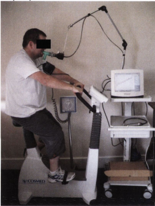
Figure 3.3. VO 2 max testing apparatus, featuring an Ergoselect bicycle ergometer and Innocor metabolic analysis system.
