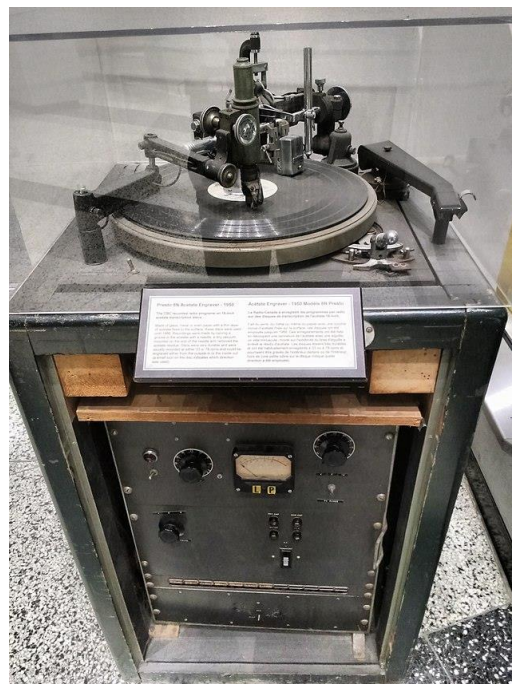
Presto 8N acetate disc engraver used by the Canadian Broadcasting Company, 1950 (Wikipedia Creative Commons)
