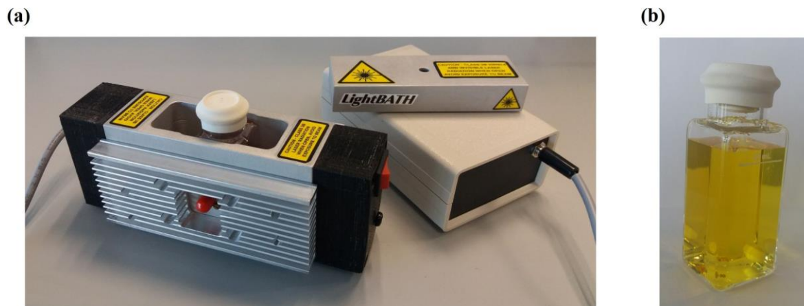
Figure 3.2. (a) LightBATH-405 advanced laser photoreactor manufactured by the UCM Optical Chemosensors & Applied Photochemistry Group (GSOLFA) of Universidad Complutense de Madrid (UCM) and used for photoproducing the photoadduct 43 . (b) Optical glass bottle reactor containing the photoreaction mixture.
