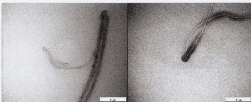
Figure 2.25 TEM images of MWNT-silica composites Silica can be seen coating the tip of the tube
