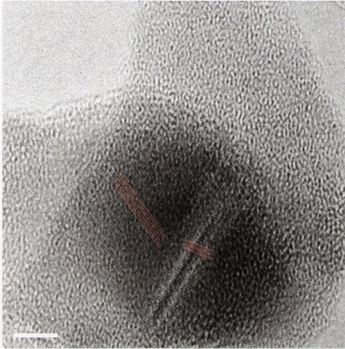
Figure 4.15: HRTEM image showing different lattice planes in a single crystalline sphere of Sample A.
