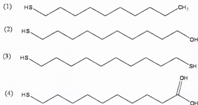
Figure 1.20: Some frequently used compounds for SAMs. For purpose of illustration, chain length is specified to n = 10 . (1) n -alkanethiol: \text{HS}-(\text{CH}_2)_{n-1}-\text{CH}_3 ; (2) \alpha,\omega -alkanedithiol: \text{HS}-(\text{CH}_2)_n-\text{SH} ; (3) \omega -mercaptoalkanol: \text{HS}-(\text{CH}_2)_n-\text{OH} ; (4) \omega -mercaptoalkane carboxylic acid: \text{HS}-(\text{CH}_2)_{n-1}-\text{COOH} ; 46
