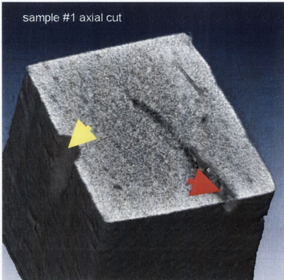
Figure 5.17 Three dimensional axial reconstruction of the bone immersed in an aqueous solution of 160. Scratch can be seen on the left side (yellow arrow). The top of the axial plane shows a vessel canal (red arrow) within the bone tissue.
