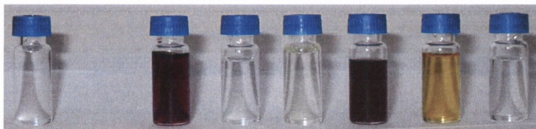
Figure 4.10 - Colorimetric effect upon addition of excess TBA salts of anions to DMSO solutions ( \sim 10^{-3} M) of 125 ; left to right: free host, F^- , Cl^- , H_2PO_4^- , HP_2O_7^{3-} , AcO^- and NO_3^-
