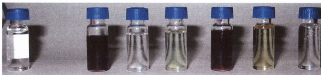
Figure 4.26 - Colorimetric effect upon addition of TBA salts of anions to DMSO solutions of 137 ; left to right: free host, F^- , Cl^- , H_2PO_4^- , HP_2O_7^{3-} , AcO^- and NO_3^-
