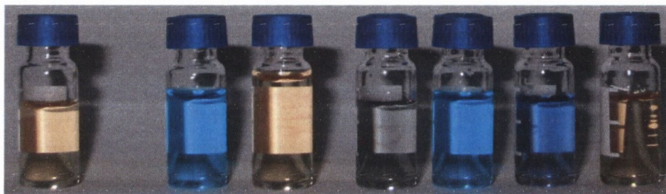
Figure 4.33 - Colorimetric effect upon addition of TBA salts of anions to DMSO solutions of crude 139 ; left to right: free host, F^- , Cl^- , H_2PO_4^- , HP_2O_7^{3-} , AcO^- and NO_3^-
