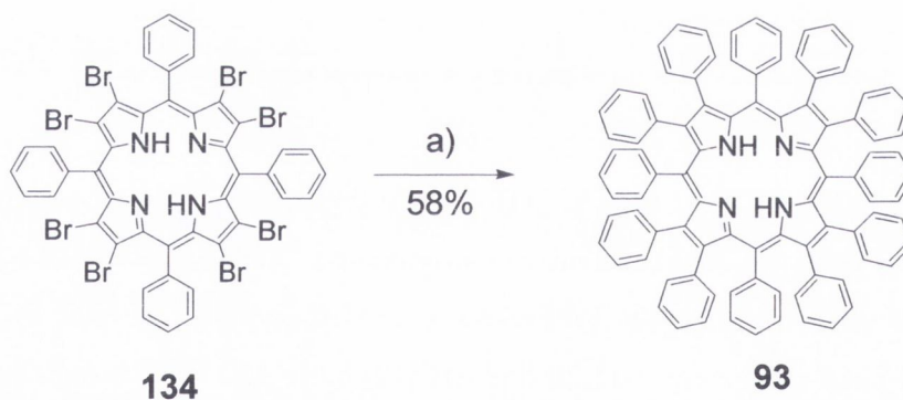
Scheme 1.5.1. Suzuki coupling reaction yielding dodecaphenylporphyrin 93 (DDP); PhB(OH) 2 (20 equiv.), K 2 CO 3 (40 equiv.), Pd (PPh 3 ) 4 (15 mol%), toluene, 7 days, 90 °C. 84
