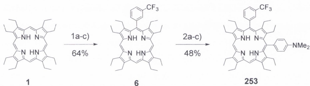
Scheme 2.2.1. Synthesis of the meso AB-substituted OEP 253 , 1a) 3-bromobenzotrifluoride/ n -BuLi in ether, -30\text{ }^{\circ}\text{C} to rt for 3h, 1b) addition of OEP 1 /THF, -30\text{ }^{\circ}\text{C} to +50\text{ }^{\circ}\text{C} , 40 min, 1c) H 2 O, then DDQ/CH 2 Cl 2 , -10\text{ }^{\circ}\text{C} ; 2a to 2c) in similarity to 1a) to 1c).
