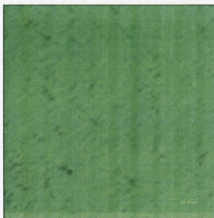
Figure 4. CLSM image of a typical section of hydrogel incorporating 0.05% w/w 2 , showing the homogeneity of the sensor within the hydrogel. This image was recorded at pH 2.5.
