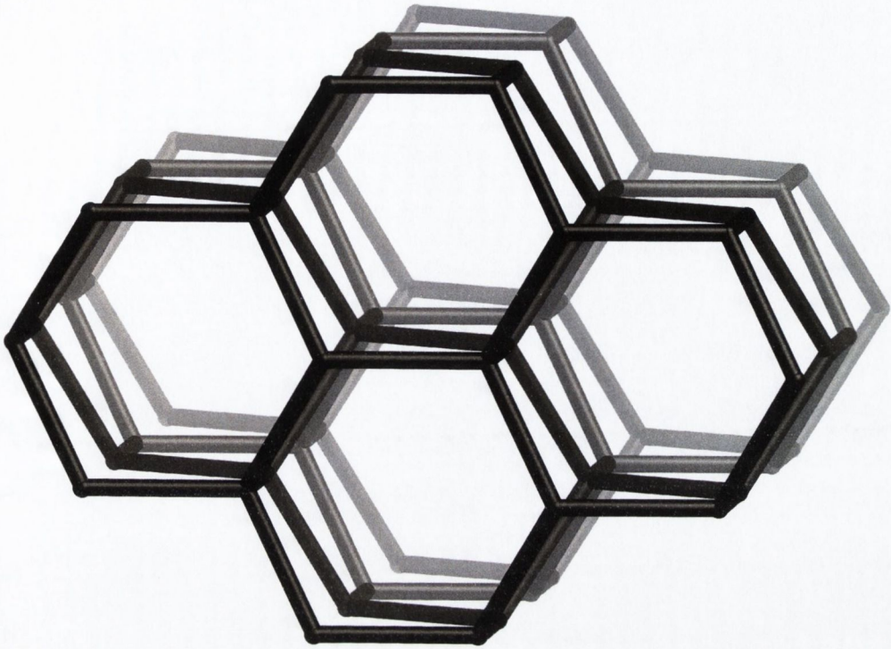
Figure A3 – Structure of lonsdaleite, consisting of four-connected nodes.
