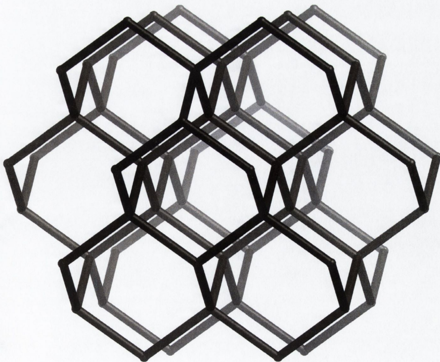
Figure A2 – Structure of diamond, consisting of four-connected nodes.
