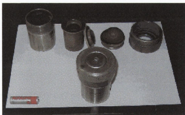
Fig 6.1. Photograph of the working components of the Bomb (Back Row) and the bomb as it appears when sealed (Front row). The Teflon insert is second from the left in the back row. AA Battery is used as scale.
