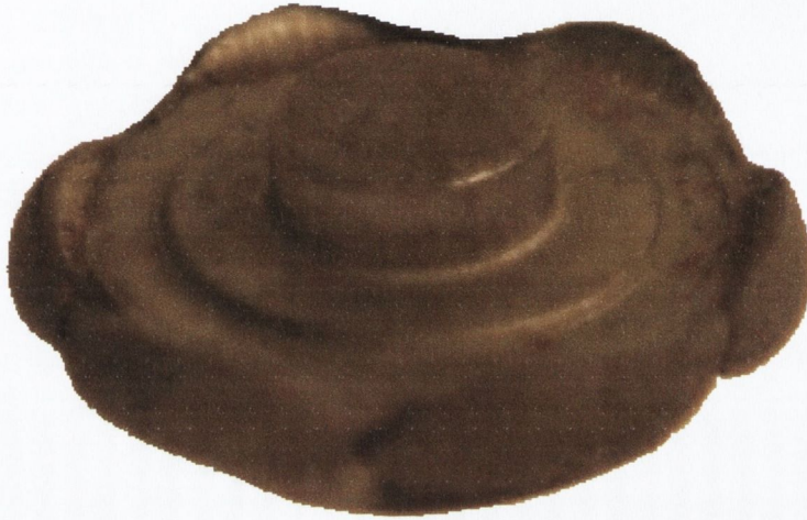
Figure 4-95: Actual Bolt Head Showing Excess Trimmed Material.
