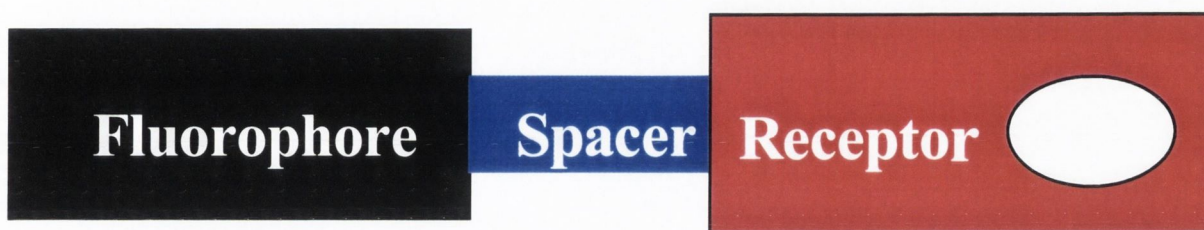
Fig. 1.3: Example of the structure of a sensor, in this case a PET sensor (discussed fully in chapter 4)
