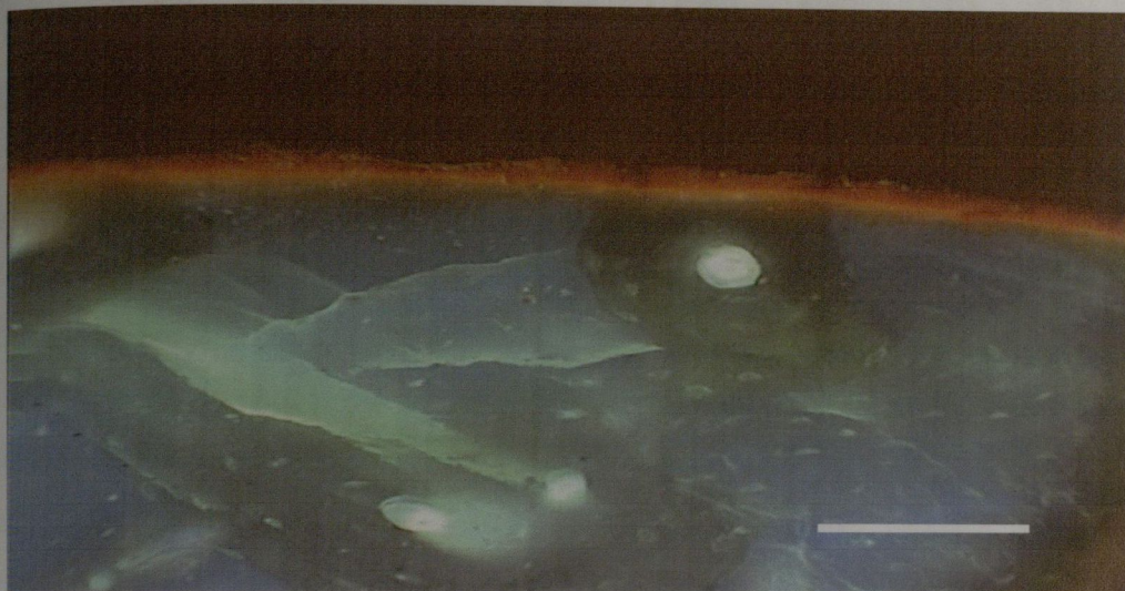
Fig. 2.6 Section through fatigue- tested specimen viewed using UV epifluorescence. Alizarin (red), which was applied prior to testing can be seen on the surface of the bone while calcein (green) which was applied during the test can be seen to label microdamage. Bar=100 \mu\text{m} .
