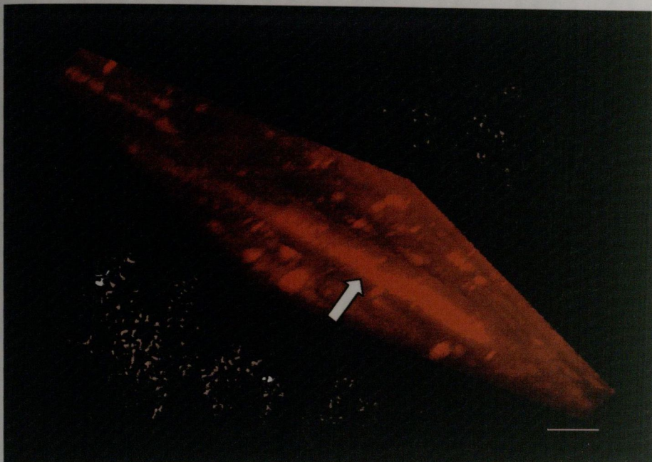
Fig. 5.7 Reconstructed microcrack obtained from dataset of images (Fig. 5.6). The crack has been rotated to show its three-dimensional shape. Bar, 50 \mu m.
