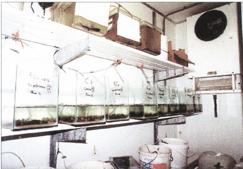
Figure 3.2. Experimental design of the in vivo laboratory exposure of zebra mussels to NP. Mussels were maintained in 12 glass tanks (control, solvent control, 5 \mu\text{g l}^{-1} and 500 \mu\text{g l}^{-1} NP in triplicate) in a climate controlled room for 112 d.
