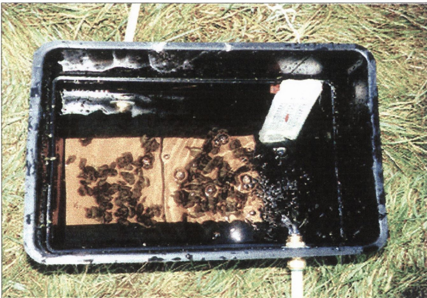
Figure 3.1. Experimental set up of in situ exposure of zebra mussel to tertiary treated effluent in Athlone STWs. (a). Effluent pumped from an effluent well into a large 135 l header tank and fed by gravity into 3 smaller 18 l plastic tanks containing the zebra mussels. Continuous flow experiment with effluent released onto the grassy area. (b). Mussels attached to tiles exposed to a continuous flow of tertiary treated effluent. Note max/min thermometer to record temperature in the tank.
