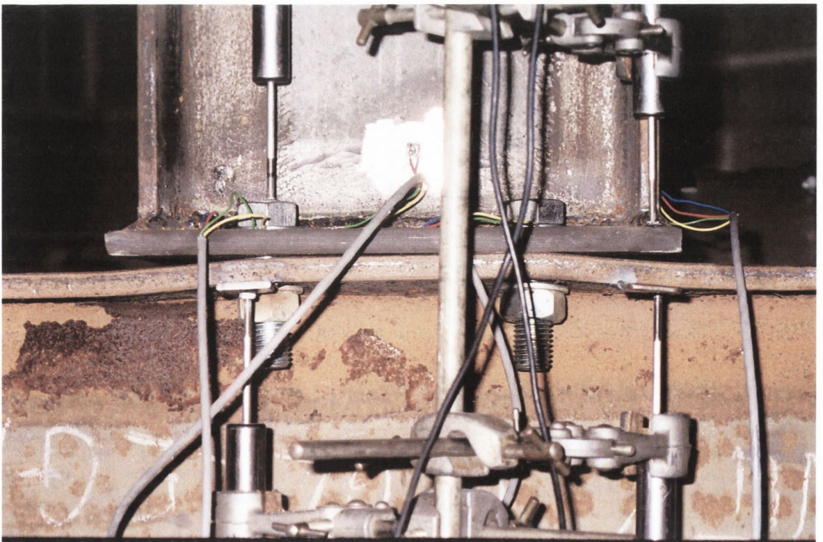
Figure 5.31: Final deformed shape of specimen 3.5
