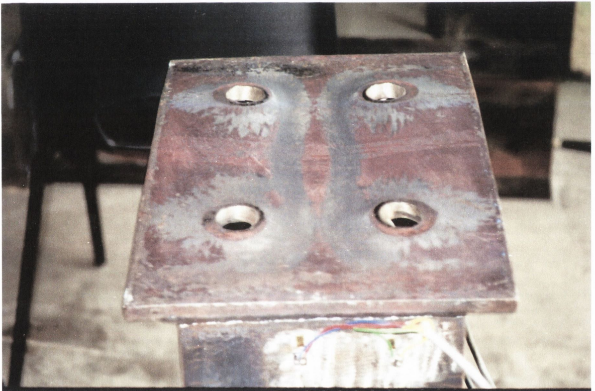
Figure 5.26: Underside of specimen 3.3 showing yield pattern
