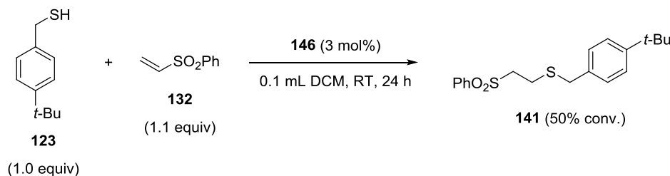
Figure 36. Optimized conditions (subsequently referred to as ‘concentrated standard conditions’) for the sulfa-Michael addition between 123 and 132 . Initially, 146 was used as a first benchmark organocatalyst. [137] a See Experimental for a general procedure. b Conversions were determined by 1 H NMR spectroscopy using dibromomethane as internal standard. c [ 146 ] = 7.1·10 -2 M.
