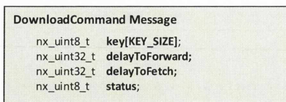
Fig. 5.12: TT - DownloadCommand Message Structure (Communication between the Vuze TT Plugin Gateway Application and the Sensor Node for Fetching and Forwarding decisions.)
