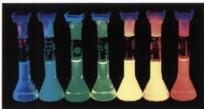
Figure 1.8: Photograph showing the effect of increasing quantum confinement/ decreasing particle size (right to left) and the resulting blue shifted, higher energy emission. Adapted from literature 45 .
