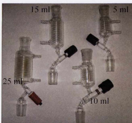
Figure 3.31. Jacket glass coil with different internal volume
