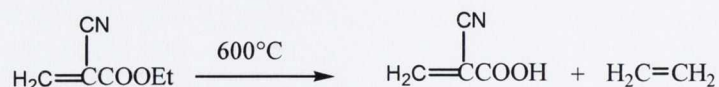
Figure 1.13 Thermolysis of ethyl cyanoacrylates for the preparation of free cyanoacrylic acid, Gololobov 47
