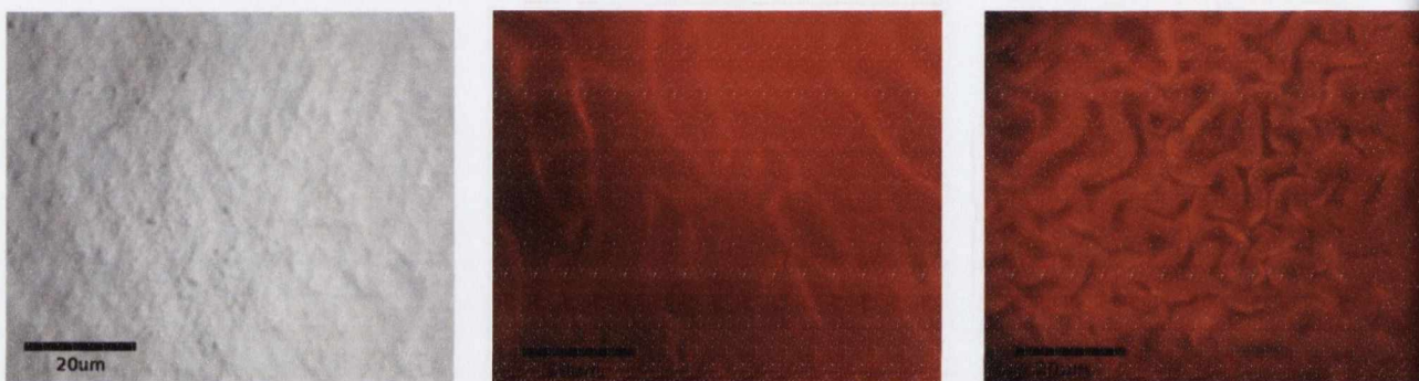
Fig. 5.15 Pure VHB elastomer (left), after swelling in CdSe/CdS QD/toluene solution for 12 hours (middle), and after swelling in QD solution for two days (right) under UV light.
