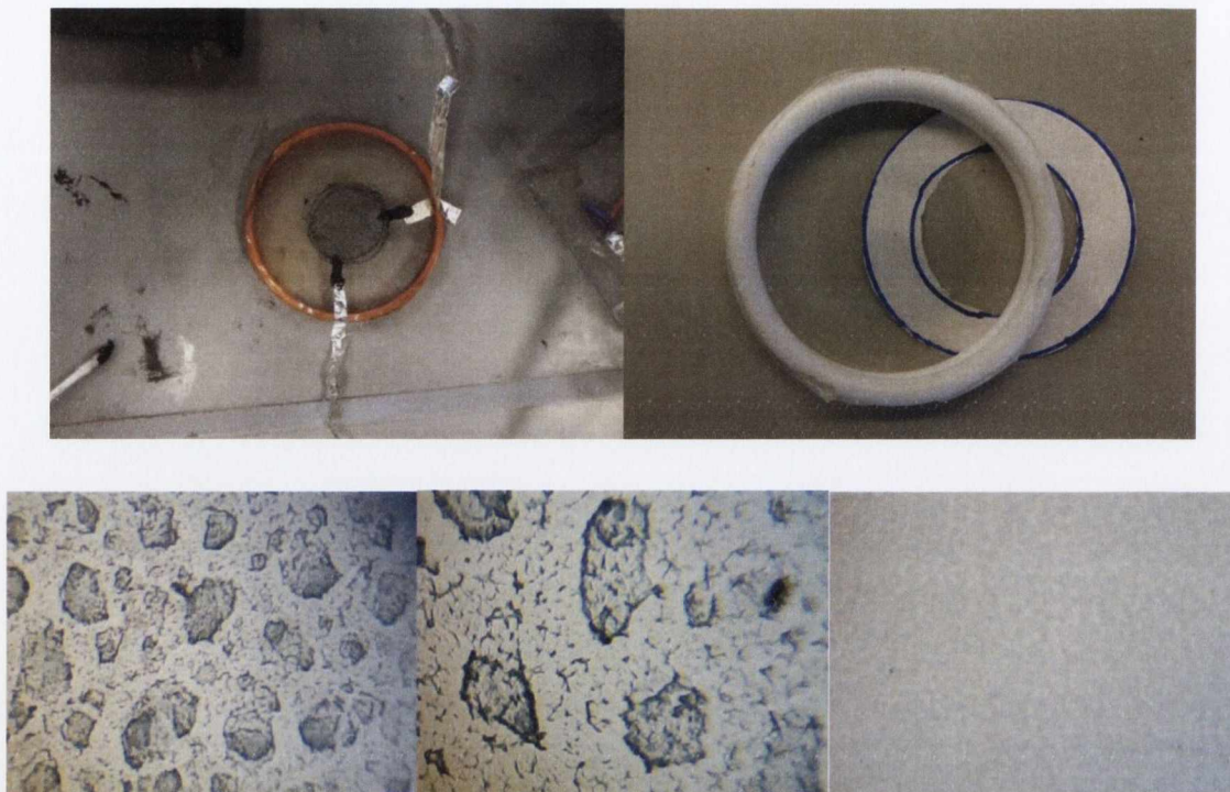
Fig 5.5. Comparison between air dried PEDOT:PSS electrode and spray dried (top, left and right) and 10x magnification of PEDOT:PSS without a heated substrate (bottom, left), air dried overnight (bottom, centre) and spray dried (bottom, right)
