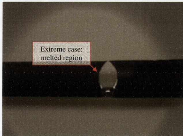
Fig. G.2: Due to the architecture of a 10 mm wide cantilever sample, a large amount of power is required to achieve the desired temperature at the extremities of the heated area. Under these conditions there is a high probability of melting at the central region, due to superior radiative and bombarding power at this zone. This event is not conducive to experiments; however, reducing the sample width improves the situation dramatically.
