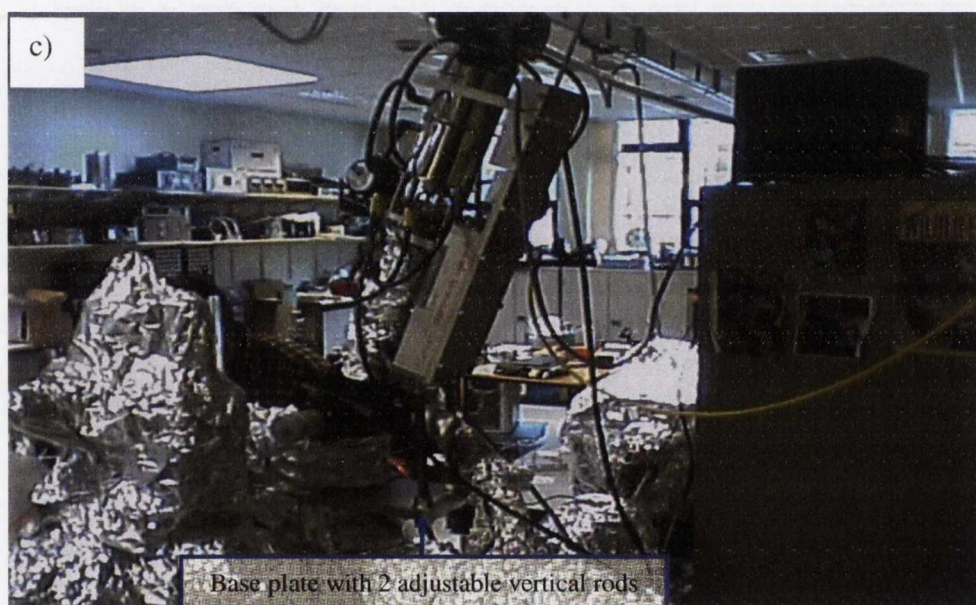
Fig. 6.18: Configuration of the infrared heating system: a) schematic diagram [42]; b) external-view during heating process; c) specifically designed support structure for the infrared heating unit to facilitate unimpeded STM and capacitance measurements.
