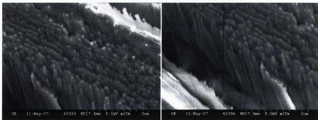
Figure 4.1: Optical Microscope (top) and SEM images (bottom) of polystyrene nanowires
