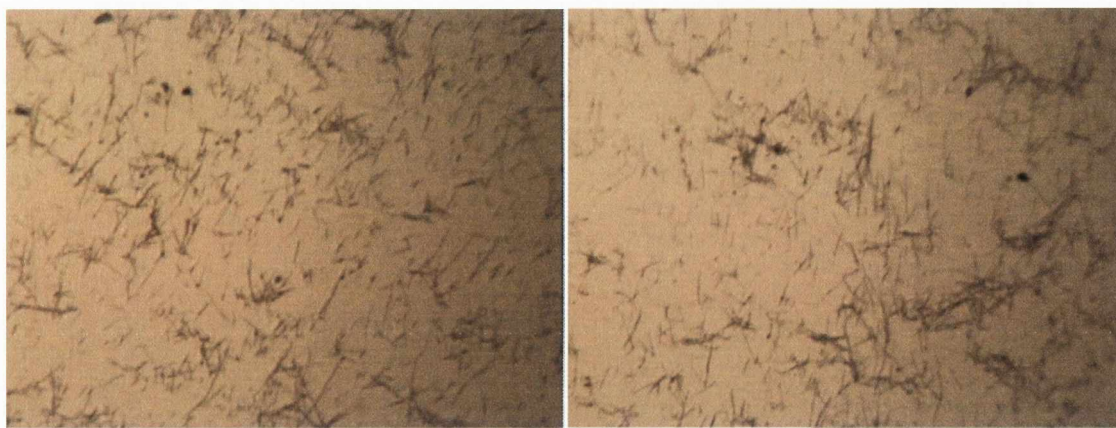
Figure 3.19: Optical microscope images showing wires in magnetic field
