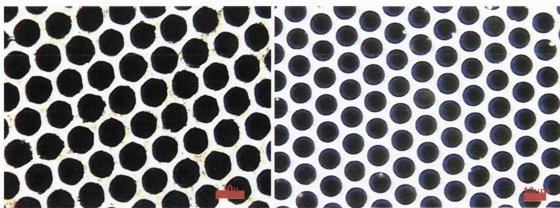
Figure 2.1: Optical images of MCG membranes with different pore diameters
