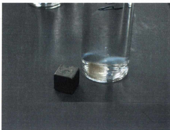
Figure 4.9: Image showing wires having been pulled through solution by magnet
