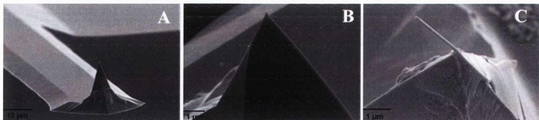
Figure 2.2: Scanning electron microscopy analysis of AFM Tips. (A), (B) and (C) are the pristine bare silicon nitride tips, tips with metal coating (Pt/Cr) and solid metal needles (silver/gallium) attached to a silicon nitride base respectively.
