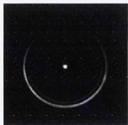
Figure 5-18: FIP of cascade ICR for linear polarised light with \Delta\gamma = 80^\circ with a ring diameter of 8.5 \times 10^{-4} m.
