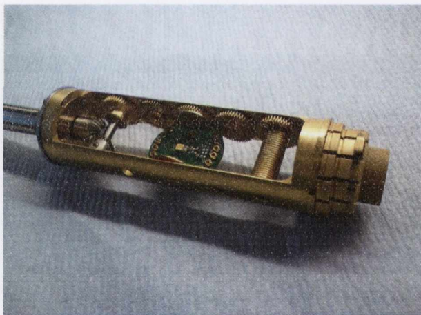
Figure 4.12: Sample rotator used for the angular dependence measurements of magnetoresistance.
