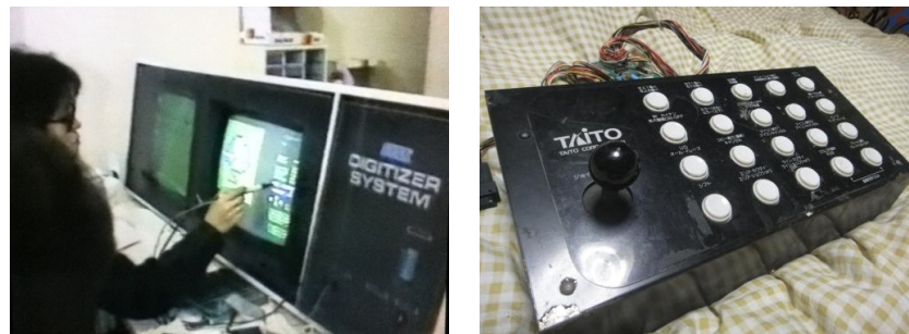
(a) Sega Digitizer used to create art-work for Fantasy Zone (1985). (b) Taito TAECOM-11 joystick interface (circa 1985).
