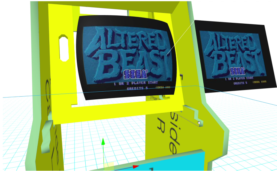
Figure 87: A live feed from Altered Beast (Sega, 1988) streamed to the HTML Canvas. The video texture is mapped to a modified sphere on the left, and to a flat plane on the right.
