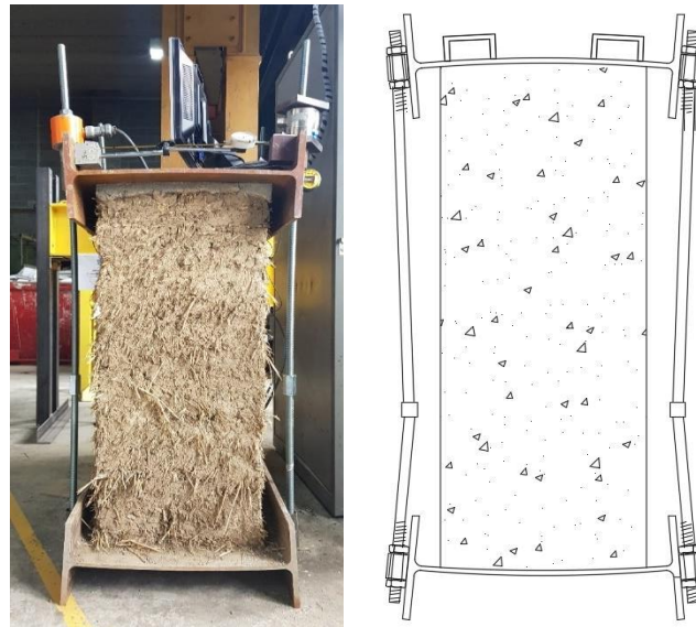
Figure 5. 37. Bending deformation on bottom steel pallet and top steel cap.
