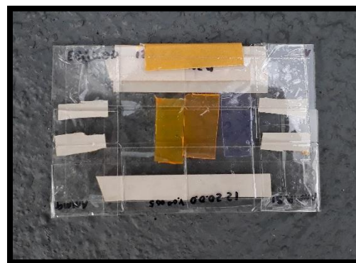
Fig 2: Samples placed outdoors in holder with window on top. L-R: PMMA, Yellow, Orange, and Violet
