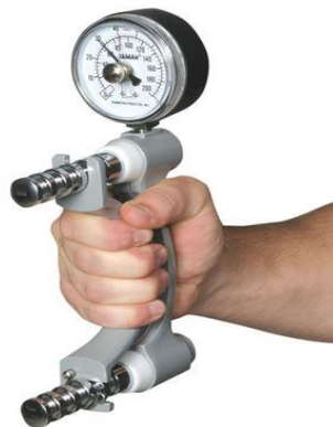
Figure 4. 1 Handgrip strength assessment using a Jamar dynamometer
