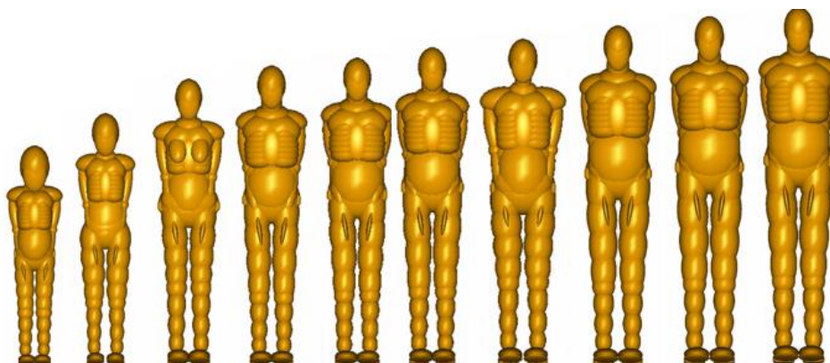
Figure 8.4 MADYMO pedestrian models, 3 years old, 6 years old, 5% percentile, 160cm (scaled), 170cm (scaled), 50% percentile, 180cm (scaled), 95% percentile and 190cm (scaled), from left to right.
