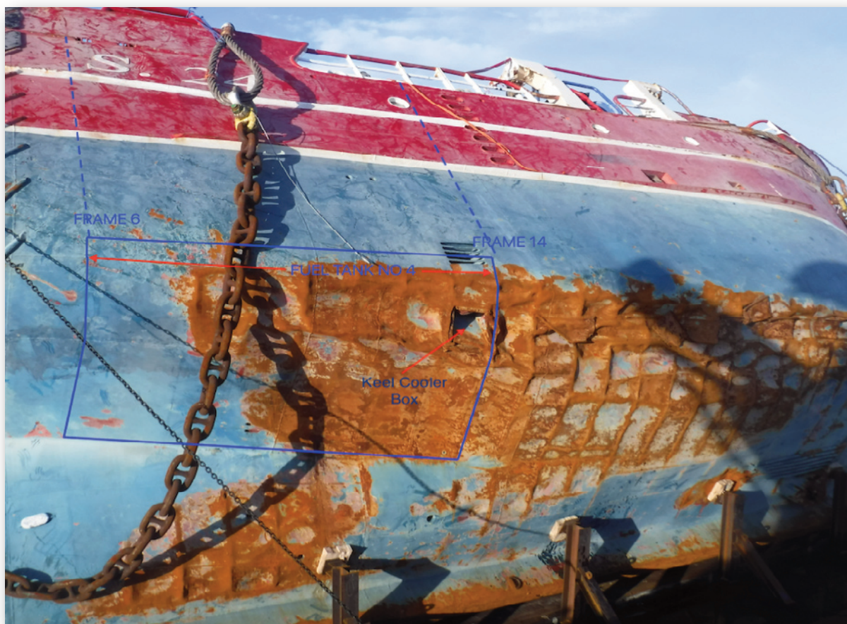
Photograph No.3 - Position of No.4 fuel bunker tank located between frames 6 to 14.
