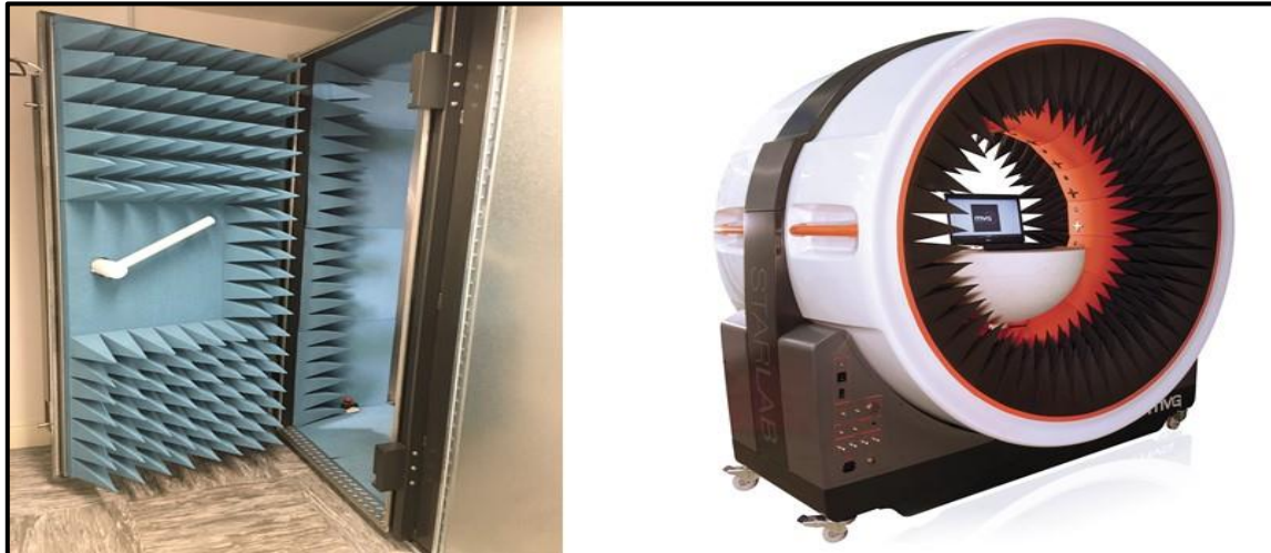
Figure 2: MVG StarLab Measurement System on the right was placed inside the Anechoic Chamber on the left for TRP and TIS Measurement 18
